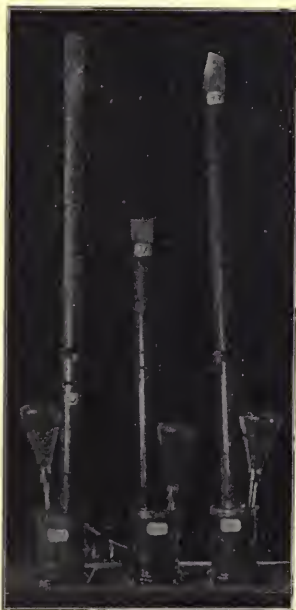
FIG. 54. The Capillary Water of Soils.
